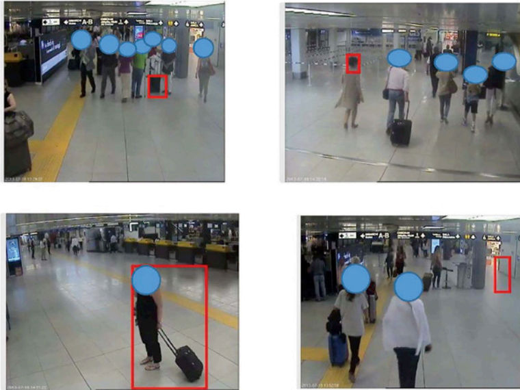
Figure 9. The image shows the failure of the software detection system, mistaking a body for the floor, a bag separated from its owner (though it is not), or the wall as a moving entity. Permission from Daniel Neyland.
